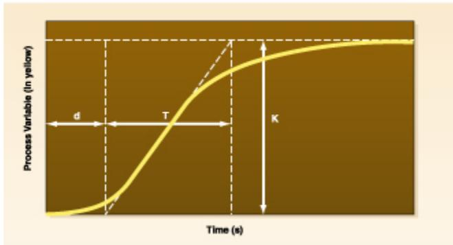
An open-loop step test reveals the process' time constant  $T$ , deadtime  $d$ , and gain  $k$ .
