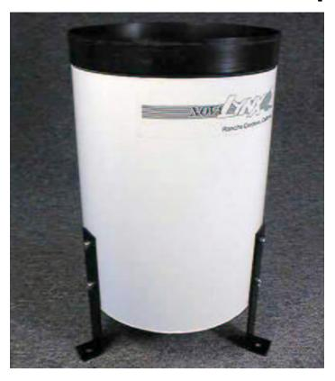
This tipping bucket rain gauge provides inexpensive, accurate rainfall measurement. Precipitation is collected in the funnel and measured by the calibrated tipping bucket.
