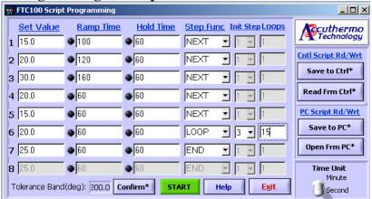
**Set Value** – is the set point temperature (in °C) for a given step and ranges from -50°C to +150°C and can be entered to tenths of a decimal.
